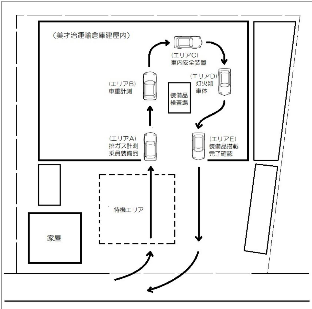
waiting zone – A(emission check) – B(weighing) – C(Safety) – D(Lamps) –E(Equipment)
